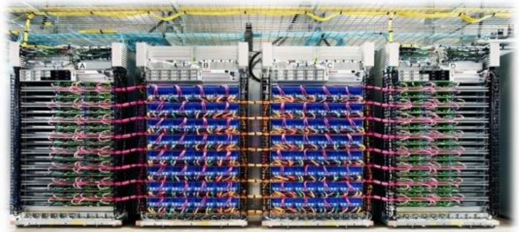
Google Cloud TPU Pod = 64 Cloud TPUs = 11.5 PFLOPs of compute!
